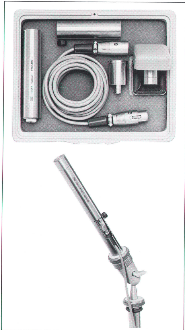
Fig. 3. Loudness analyzer microphone consists of 1" condenser microphone cartridge and preamplifier. Response is flat within \pm 1 dB from 30 Hz to 8 kHz and within \pm 2 dB from 8 kHz to 18 kHz.
